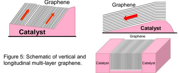
Figure 5: Schematic of vertical and longitudinal multi-layer graphene.
