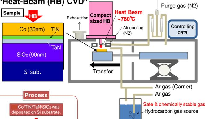
Figure 2: Heat-Beam CVD machine.
