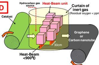
Figure 1: Roll-to-roll system using HB.
